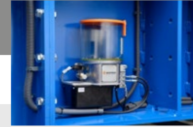
Lubrication Central lubrication during operation
