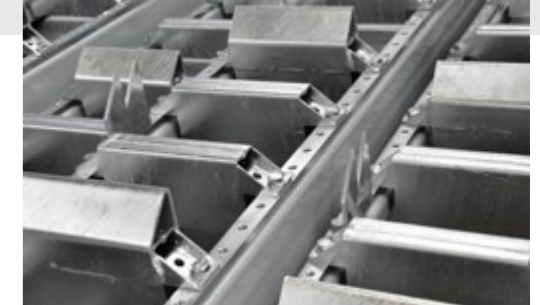
Feature Special paddle adaptation for optimised separation of cardboard
