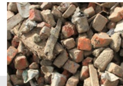
Landfill extraction 2-stage separation: screen 90–200 mm
