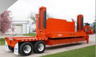
C&C Impact 5 Revolutionary Quad-Post Guide System The key to the Quad-Post system is the equal distribution of the crushing force to the four corners of the crushing lid. The crushing lid is connected to the four sliding guides by heavy-duty pivot lugs mounted on each corner. The stress is distributed equally across the guide posts, sliding guides and pivot lugs, giving the Impact 5 greater stability and durability.
