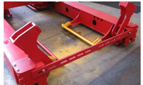
Container rests raised
