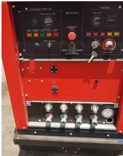
Fig.4: Colour coded hydraulic hoses
