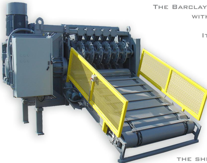
THE BARCLAY 4.9 PRIMARY SHREDDER WAS DESIGNED WITH THE PURPOSE OF BEING THE FIRST AND FOREMOST CUT IN ANY SHREDDING LINE. IT IS CAPABLE OF CUTTING RIM FREE TIRES RANGING IN SIZE FROM PASSENGER TO SUPER SINGLE TIRES.
