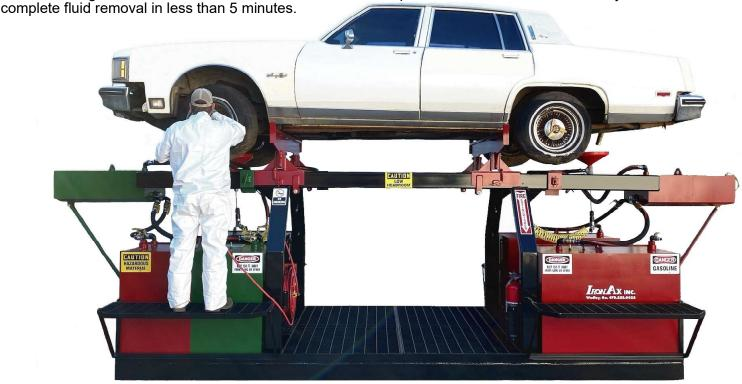
The Enviro-Rack pictured is equipped with a gasoline separation system, antifreeze separation system, and fold out catwalks.
