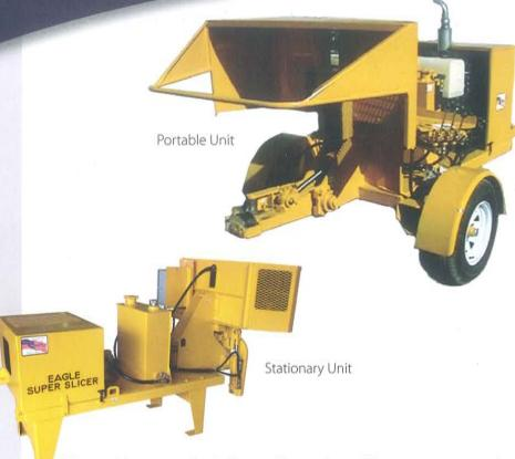
The multi-purpose Eagle Super Slicer unit enables you to remove the sidewalls or the steel beads from truck tires, light truck tires and car tires. The cycle time is twelve seconds on truck tires (up to 44" outside diameter) production rate of 50-60 per hour, and eight seconds on car tires (13" to 16" outside diameter) production rate of 70-90 per hour.
